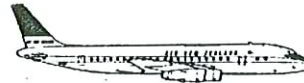
Douglas DC-8 série 52 (Douglas Aircraft Co, USA) 155 pax, 2 pnt, 8 pnc 870 km/h 7 appareils/1968-1989
