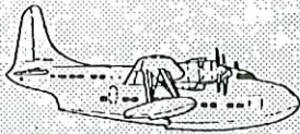
Short S.45 Solent Mk III (Short Bros, UK) 39 pax, 5 pnt, 3 pnc 300 km/h 4 appareils/1949-1960
